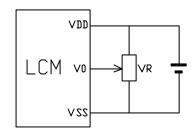
VDD~V0: LCD Driving voltage
